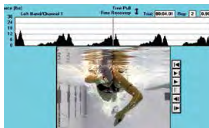
FIG. 1 > (ABOVE) These images show three female freestylers and the force curves for their left hand. The vertical gray line on the force curve is synchronized with the video image.
